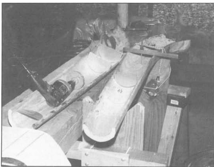
Carving and hollowing the cedar alphorn
