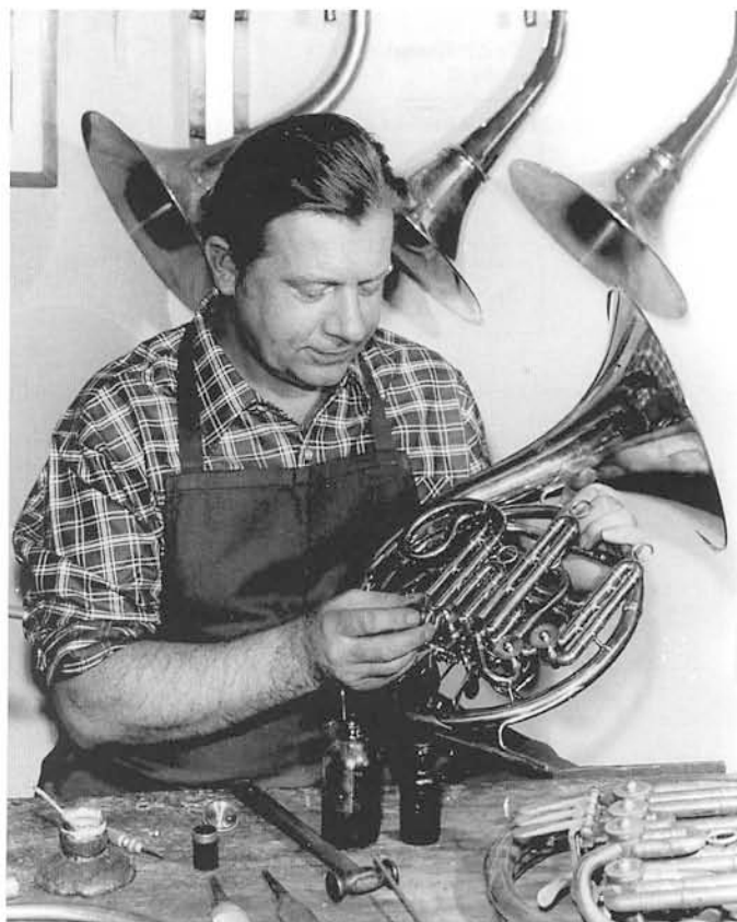
Johannes Knopf (1929-1981) in his workshop, about 1970(?). He is working on a Knopf Model 14, F/Bb compensating double horn with an E-A/stop valve. On this model, the slide has to be pulled out for stopping on the Bb side.
