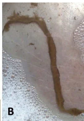
Fig. B – Massive amount of material from leadpipe, unknown when last cleaned.
