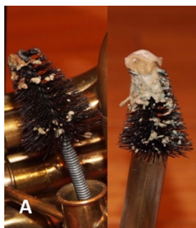
Fig. A – Leadpipe cleaned 5 weeks previously (left), neglected main tuning slide (right).
