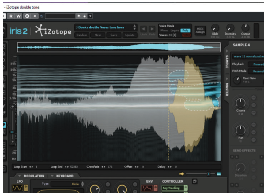
Figure 7. Another tiny portion of the sound is shown, now in Iris2. The fundamentals and overtones are white horizontal lines and the large gray and beige areas indicate volume.
